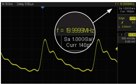
Built-in arbitrary waveform at 20 MHz, 300 MSa/s
